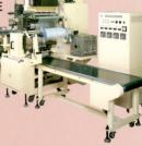
This is an automatic pouch machine designed to package single-use, easily disposed of fabric applicators. In this machine, four reels of cotton cloth in tape form are unexound, fed in parallel, cut off to length, folded and then impregnated with an anticeptic solution, while pouches are formed, filled, seled on four edges, collated and ejected from the machine as a complete towelette package.
